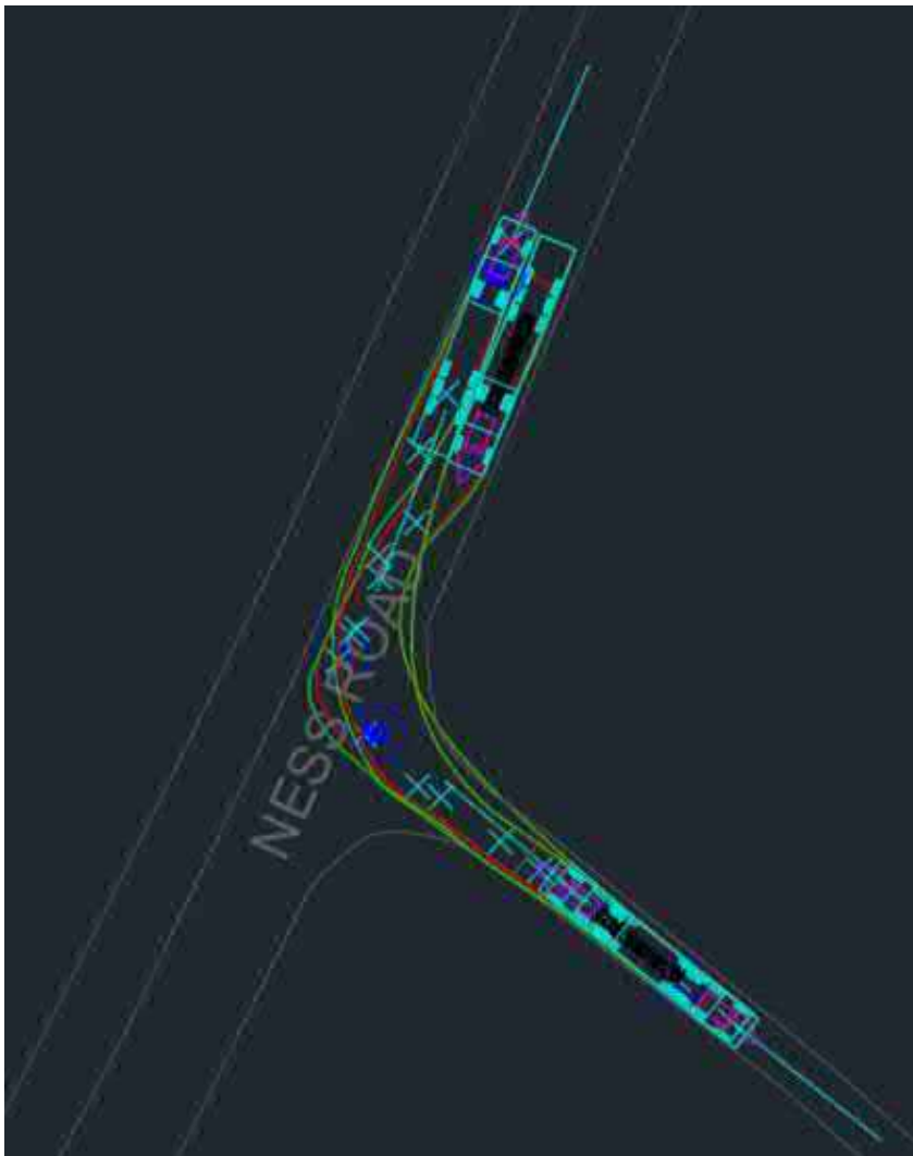
Figure 15: Ness Road – Vehicle Tracking (Entry and Egress)
