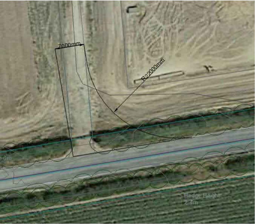
Figure 16: Crane Entry Option 2 – Junction Works Area*
