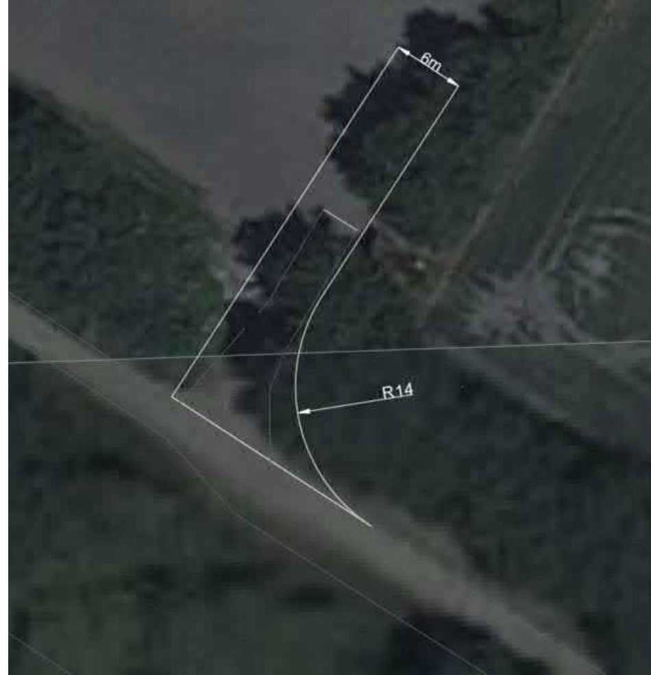
Figure 3: Option 2 – Indicative Junction Works Area
