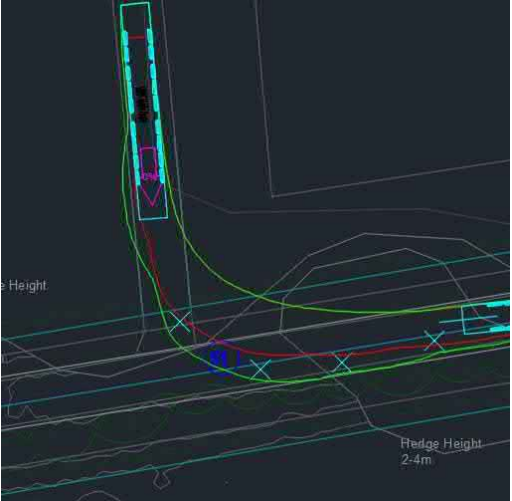
Figure 11: 1000T Crane Egress
