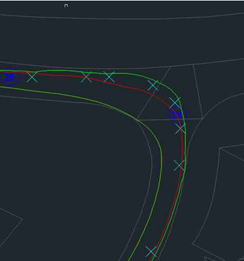
Figure 47: Swept Path Analysis: 650T Crane A11/Elms Road
