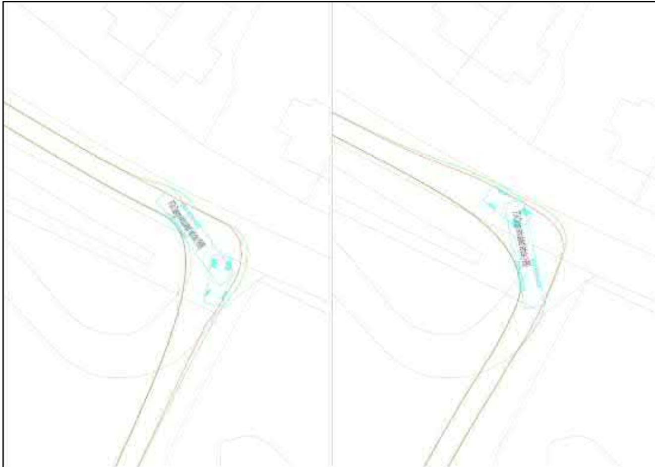
Figure 35: Sunnica West- Access C – Vehicle Tracking (Entry and Egress)
