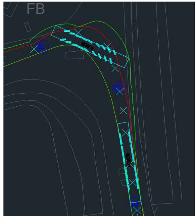
Figure 25: Swept Path Analysis – 1000T Crane – A142 Fordham Road/Windmill Road T-Junction – Egress
