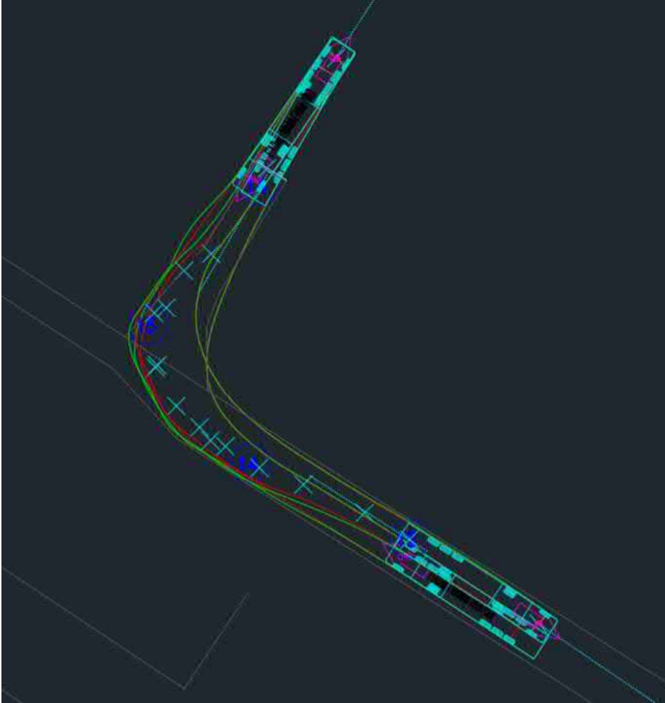
Figure 2: Option 2- Vehicle Tracking (Entry and Egress)
