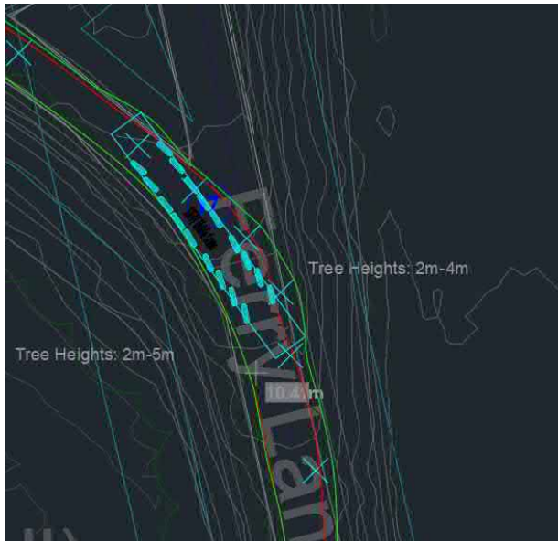
Figure 18: 1000T Crane Egress
