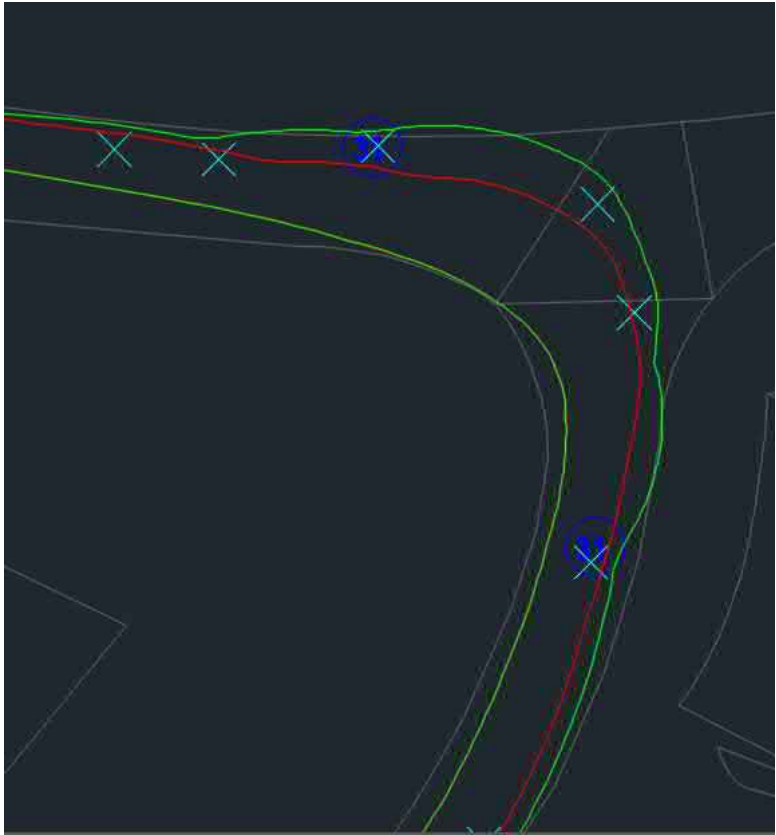
Figure 48: Swept Path Analysis: 400T Crane A11/Elms Road
