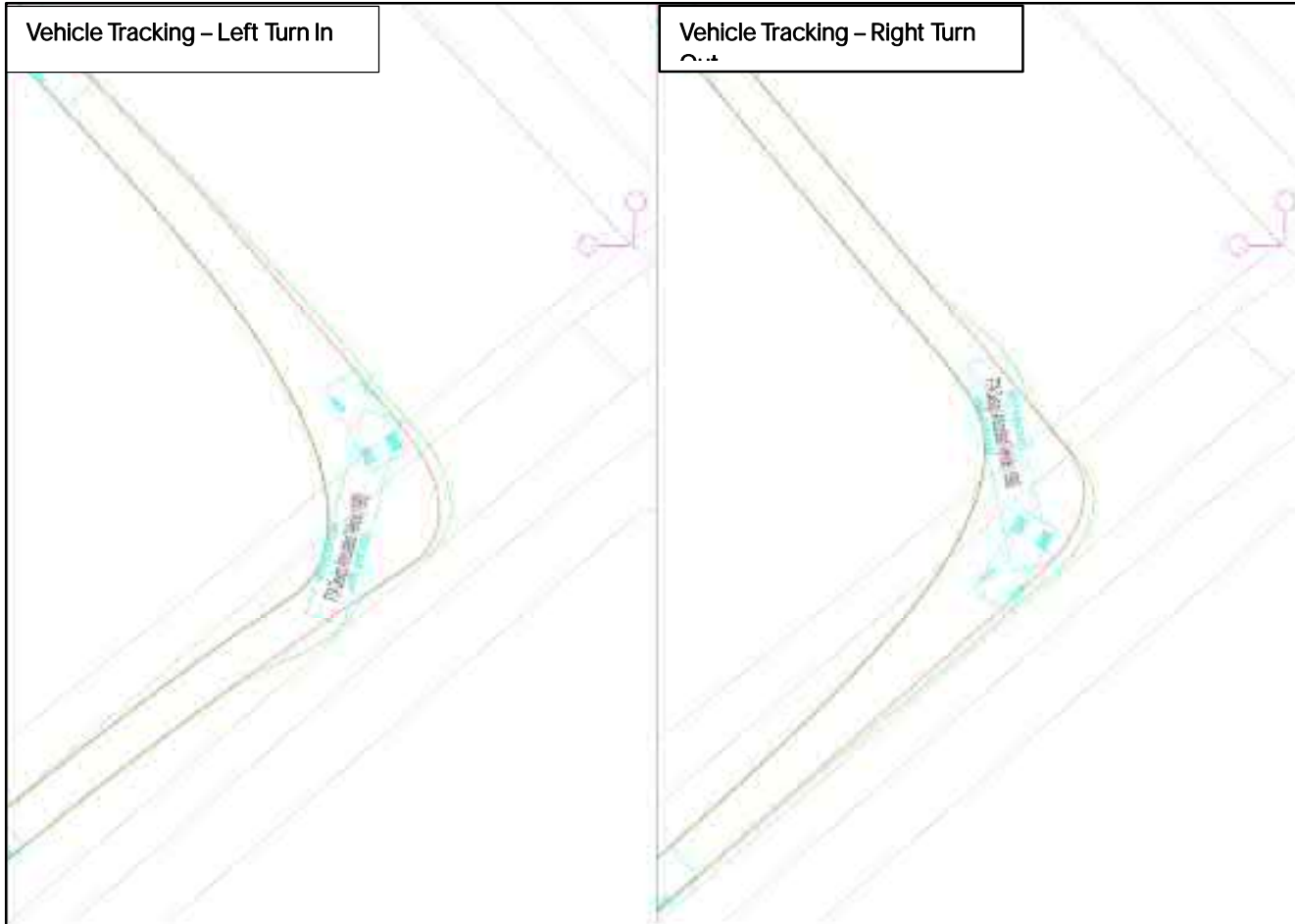
Figure 32: Cable Route Site Access M – Vehicle Tracking
