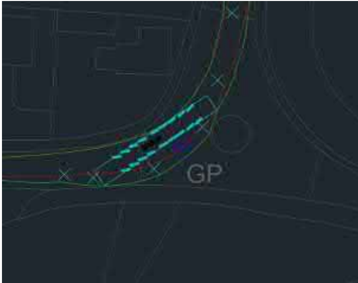
Figure 30: 1000T Crane Egress
