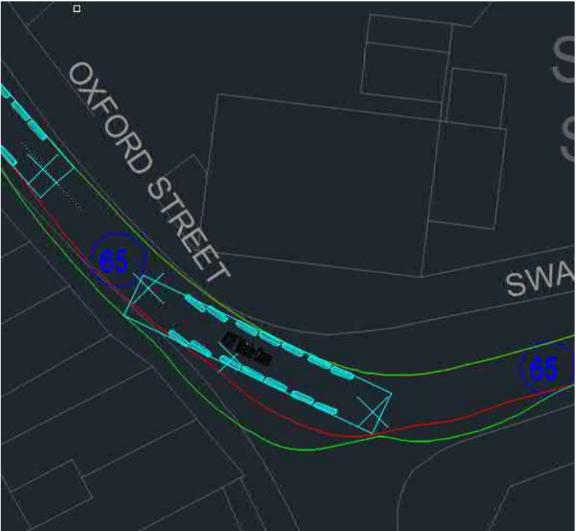
Figure 11: Swept Path Analysis: 400T Crane Entry
