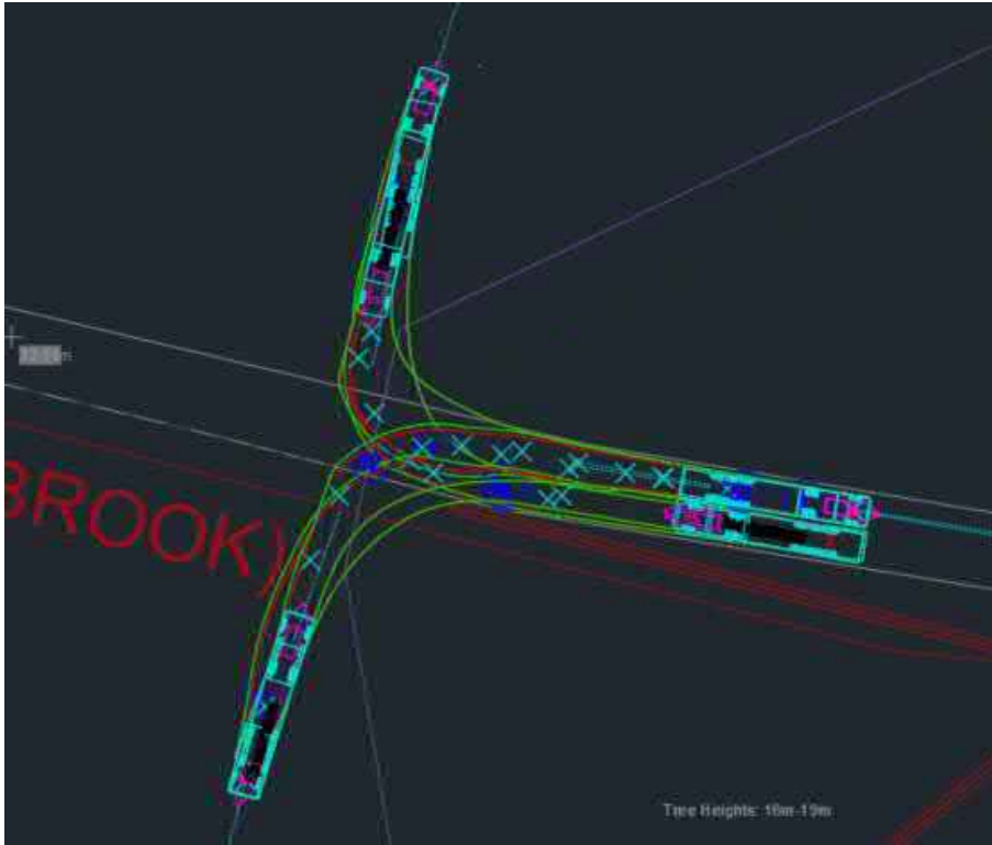
Figure 34: B1085 – Vehicle Tracking (Entry and Egress)
