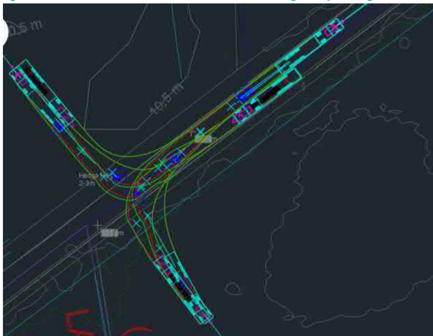
Figure 37: B1102 Freckenham Road – Vehicle Tracking (Entry and Egress)
