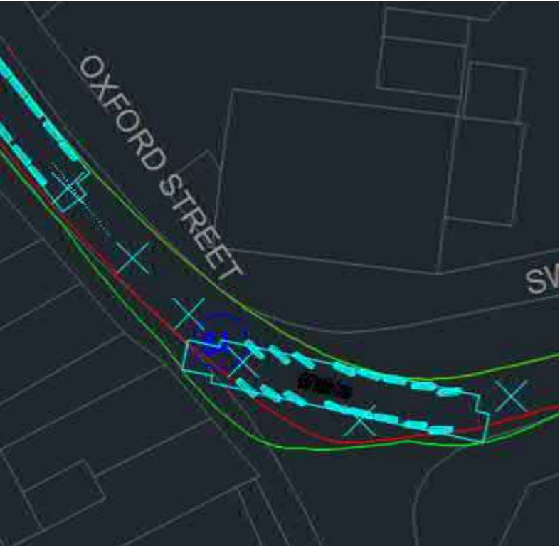
Figure 10: Swept Path Analysis: 650T Crane Entry
