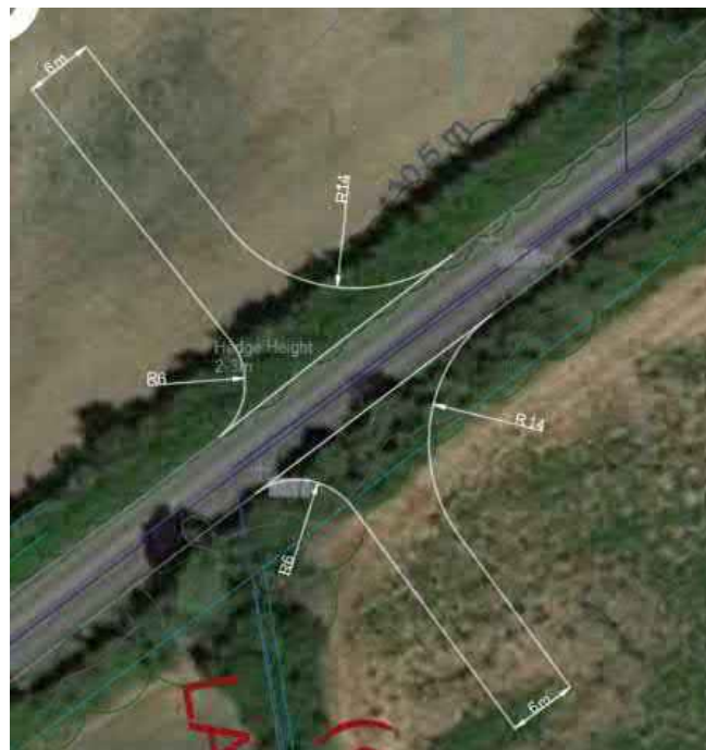
Figure 38: B1102 Freckenham Road – Indicative Junction Works Area
