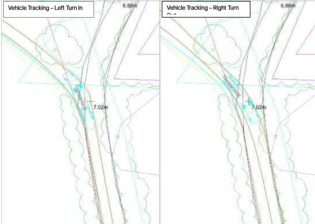
Figure 15: Sunnica East – Access E – Vehicle Tracking
