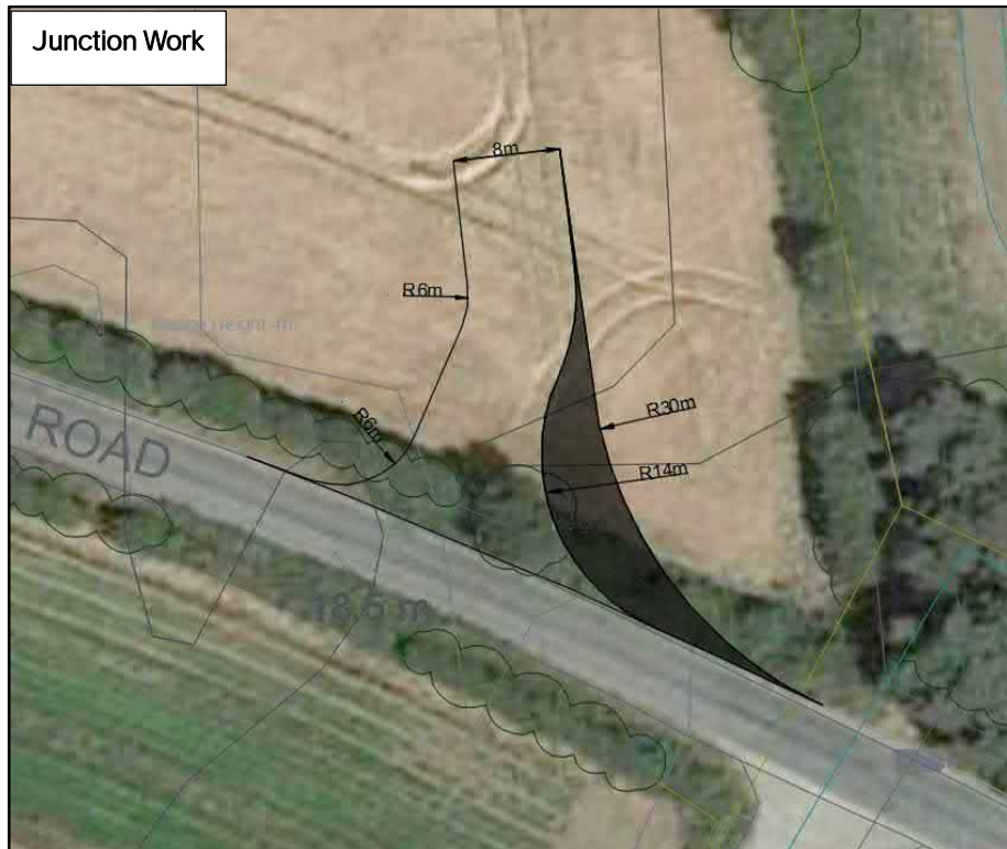
Figure 4: Sunnica East – Access A – Junction Work
