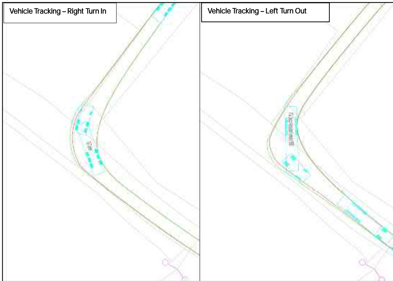
Figure 18: Sunnica East – Access F – Vehicle Tracking
