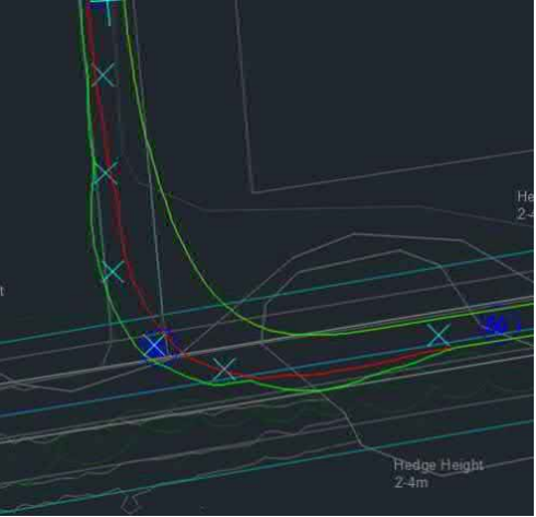
Figure 10: 1000T Crane Entry
