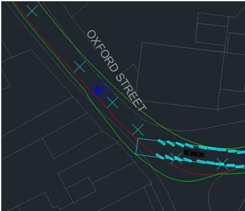
Figure 8: Swept Path Analysis: 1000T Crane Entry
