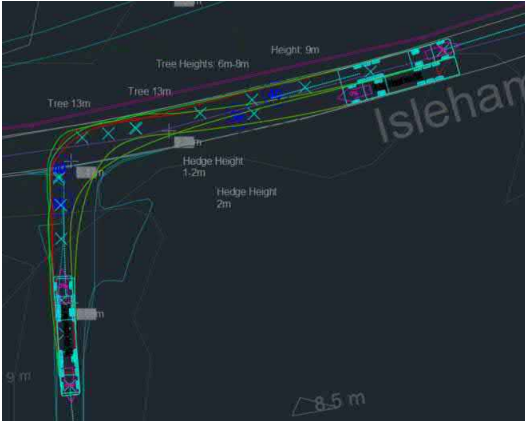
Figure 40: Isleham Road – Vehicle Tracking (Entry and Egress)
